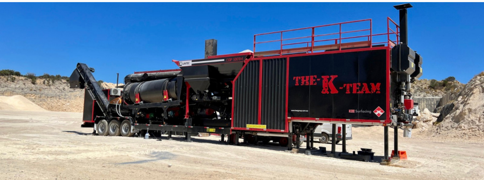
Pictured: KEE's new Lintec CDP5001M continuous asphalt mixing plant, aka "The Bandit".
